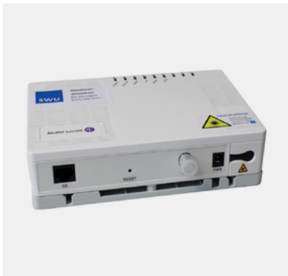
Abbildung 25: Optical Network Termination (ONT)
